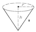
In a right circular cone, the axis (h in the diagram) is perpendicular to the base. The volume of a right circular cone is calculated using the following formula:
