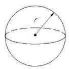
The volume of a sphere is calculated using the formula:  $V = \frac{4}{3} \pi r^3$
